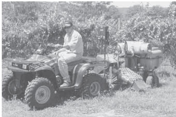
The Atarus Stinger uses a propane-fired generator to create a high velocity stream of super-heated steam which is directed at weeds.
