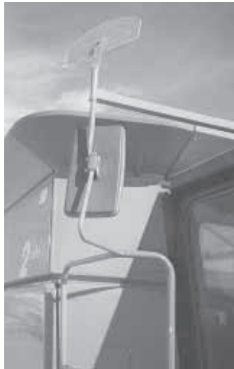
Add-on mirror mounts about 2 ft. above factory mirror on right side of combine. Mirror lets operator see down into tank so he can stop before grain spills over.
