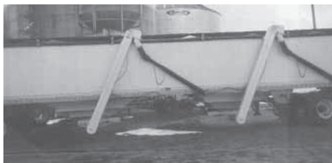
Don and Jason Jaquish save time and reduce damage to seed by filling their planter directly from the semi trailer they use to bring seed home.
