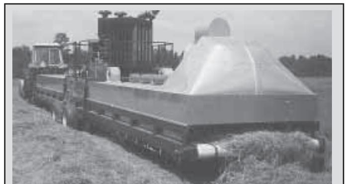
**Prototype microwave hay dryer used 210 household-type microwave units to dry high-moisture hay.**
