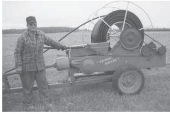
Steve Drobot designed this pipe roller to unroll and roll up water lines when moving from field to field as livestock are rotated.
