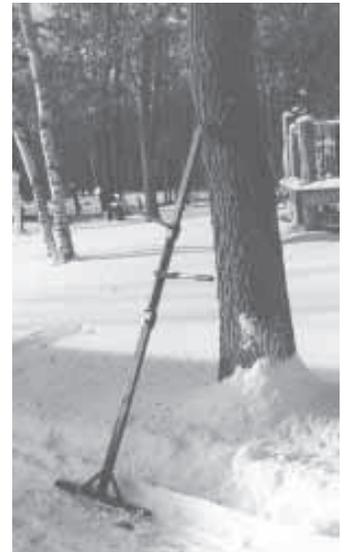
Lothe's 76-in. long "tree jack" consists of a heavy duty screw jack attached to pieces of sq. tubing. He extends the jack to push tree over.
