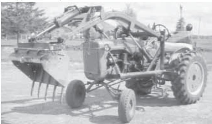
Levi Larson used side rails from the frame of an old car to make the lift arms on his front-end loader. It's mounted on his Allis Chalmers B tractor.
