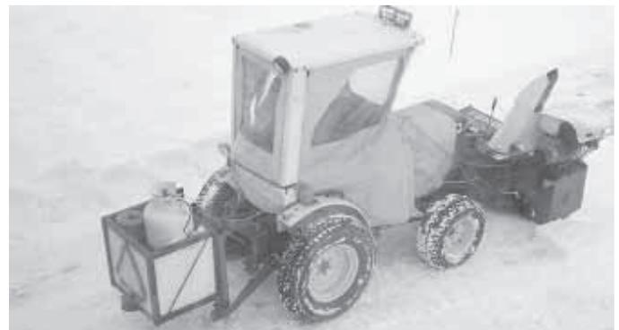
**Snowblower is belt-driven by a Honda 11 hp engine mounted directly on blower. A small air compressor and a 20-lb. propane tank on back are used to operate an air cylinder that pushes blower engine up to tighten drive belt.**
