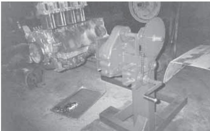
**Matt Throener of Carnegie, Okla., made his own engine stand, mounting a final drive gearbox from an 860 Allis Chalmers cotton picker on a home-built steel frame.**
