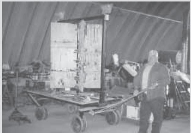
Four plywood panels hang from a steel frame. All eight sides of panels are fitted with tools.
