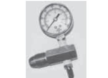
unit connects directly to the tank. After purging the propane completely from the tank, you attach the adapter and fill the tank using any standard tire inflation nozzle. The converted container works great to inflate
