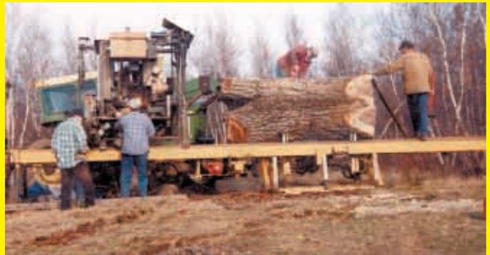
My home-built sawmill will handle the biggest, toughest logs. It's powered by a 50 hp. Cummins Onan engine, which runs the bandsaw blades and debarker. An 11 hp. Honda engine runs all hydraulics on the log carriage itself. The saw's operated by 32 switches. Our best 2-day run with the sawmill was 12,128
