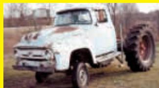
There have been a lot of trucktors built over the years. Here's a version I built back in 1983 by connecting part of a 1956 Ford 1-ton pickup to a Farmall M tractor. It's a great toy. I'm 85 years old and recently had open heart surgery, so I haven't operated my trucktor for two or three years. It gets 6 to 10 mpg. (Burdette R. Masters, Box 304, RR 3, Chariton, Iowa 50049 ph 641 862-3275)
