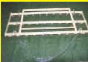
My new "Johnny Rake" is designed to recondition gravel driveways and to aerate lawns and remove thatch. It measures 48 in. wide by 20 in. long and is equipped with three rows of self-cleaning steel teeth that face backward.
