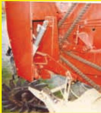
I converted the manual lift pickup on a friend's New Holland 640 "Silage Special" baler to hydraulic lift. The baler, which is about seven years old, came equipped with a standard manual lift pickup so every time my friend went over a ditch or switched fields, he had to get out of his tractor and raise the pickup up out of the way.
