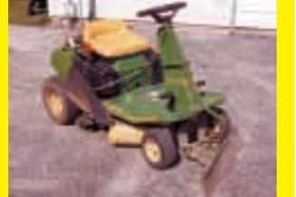
plate, measures 31 in. wide by 6 in. high. I had a local machine shop bend the blade into a curved shape and used a pair of metal brackets to attach it to the mower frame. The blade pivots up or down on a horizontal steel pin, and its side-to-side angle can be adjusted by changing the position of a pin that goes through a half-circle steel plate that's welded onto the back side of the blade. The plate has a series of holes along its perimeter.
