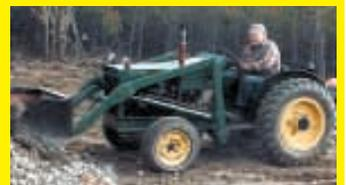
frame is made from 6-in. channel iron, and the front axle is off a Ford pickup that had twin I-beam suspension. A raised pivot point at the center allows the front wheels to move freely up or down. The steering system also came off the Ford pickup.
