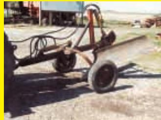
frame of the plow to act as an anchor for one end of a hydraulic cylinder. The other end of the cylinder goes to the mechanical adjustment point. The mast itself is anchored by a diagonal brace. Now it's easy to change the angle of the plow just using the hydraulic lever. **(Leon Frohn, 388 Trestle Ave., Pocahtontas, Ill. Ph 618 669-2179)**
