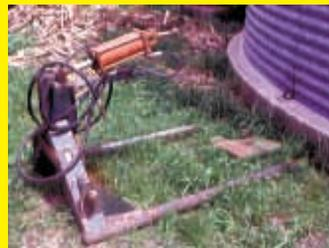
I added a hydraulic cylinder to the top link on my tractor-mounted bale fork. Gives me a lot more flexibility when handling bales. You have to have an end to go between the cylinder and the top link. **(Doug Phillips, 13438 710th Ave., Zearing, Iowa 50278 ph 641 487-7436)**
