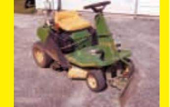
plate, measures 31 in. wide by 6 in. high. I had a local machine shop bend the blade into a curved shape and used a pair of metal brackets to attach it to the mower frame. The blade pivots up or down on a horizontal steel pin, and its side-to-side angle can be adjusted by changing the position of a pin that goes through a half-circle steel plate that's welded onto the back side of the blade. The plate has a series of holes along its perimeter.
