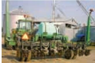
Coulter cart in front supports a pair of liquid fertilizer tanks.
