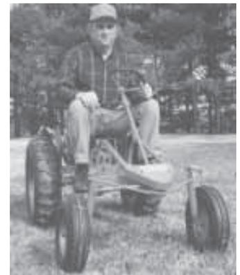
Front axle assembly was fabricated from pipe and strap iron.
