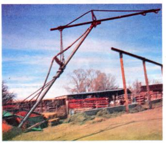
Miller built this boom out of 3-in. dia. pipe. It attaches to loader bucket with chains and is raised and lowered by loader.
