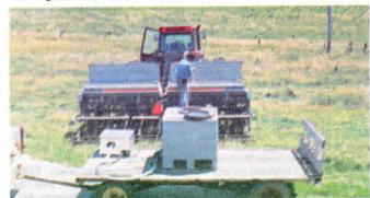
Seed blower can also be used to handle seed from a bulk seed tank.
