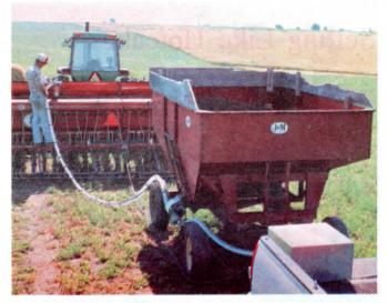
Seed blower can be attached to gravity wagon chute, letting you use air power from portable blower (sitting on pickup tailgate in photo) to quickly fill planters, drills.
