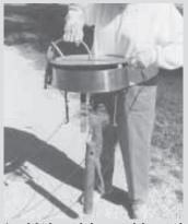
A weight hangs below a stainless steel brush inside a housing about a foot above chimney.
