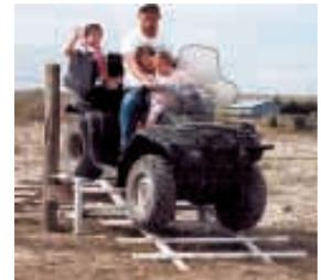
Ramps are made out of grader blade, with combine rasp bars used as cross pieces.
