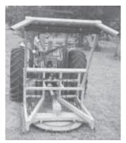
Pto-driven tree cutter is equipped with a circular 4-ft, steel blade that's pushed into tree by a pair of hydraulic cylinders. Pusher bar forces tree back away from tractor and operator.
