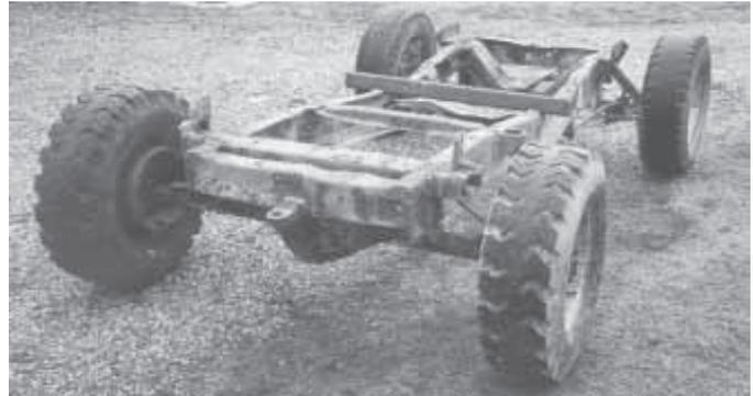
He welded steel reinforcing onto parts of pickup frame to take some load off the axles.
