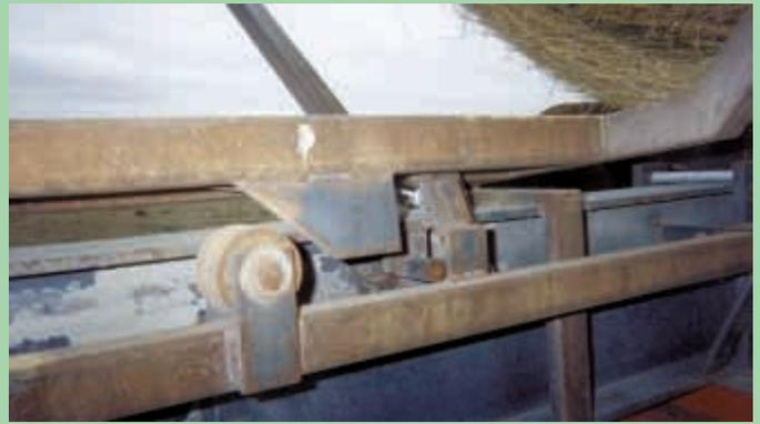
Steel tube is fitted with five rollers and five metal latches, one set for each bale cradle. They're staggered so as cylinder is extended, the tube moves back, tripping each cradle.
