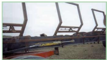
Operator controls the release of each bale by how far he extends a hydraulic cylinder, which is attached to a length of sq. steel tubing that runs along one side of trailer.
