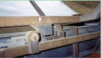
Steel tube is fitted with five rollers and five metal latches, one set for each bale cradle. They're staggered so as cylinder is extended, the tube moves back, tripping each cradle.
