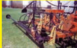
indicator lights that wire to a toggle switch. The switch bolts to a hydraulic lever that I use to control the markers. To work the markers, a main power switch is turned on, then the toggle switch is turned up and the left indicator light comes on. The hydraulic lever is pulled back and the marker is extended. To operate the other marker, you just flip the toggle switch the other way and activate the lever. (Brian Lesiuk, RR1, Gilbert Plains, Manitoba, Canada R0L 0X0 ph 204 548-2695)
