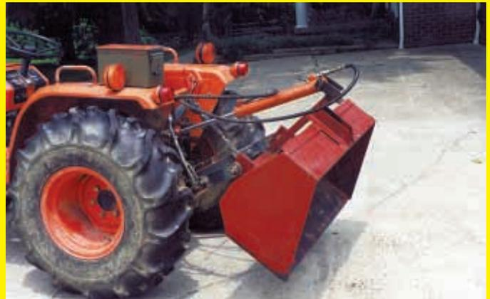
Being 75 plus years of age, I've now reached the point that it's time to use mechanical and other means to substitute for muscle power. My 19 hp Kubota 4-WVD tractor had dealer-installed hydraulics for lifting a snowblower. I simply rerouted the hoses so I could operate a custom-built, hydraulic dump bucket that mounts on the tractor's 3-pt. hitch.
