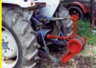
use it to power my 1920's grist corn mill. The pulley's angle shaft bolts up to the pto shaft on the rear of my older Ford tractor. I mounted it on a 3-pt. hitch system and used a pto shaft assembly from a small fertilizer spreader. I use the top link on the 3-pt. to adjust the flat belt tension. (Wayne A Beggs, 3378 Augusta Hwy., Lincolnnton, Mass. 30817 ph 306 359-1240)
