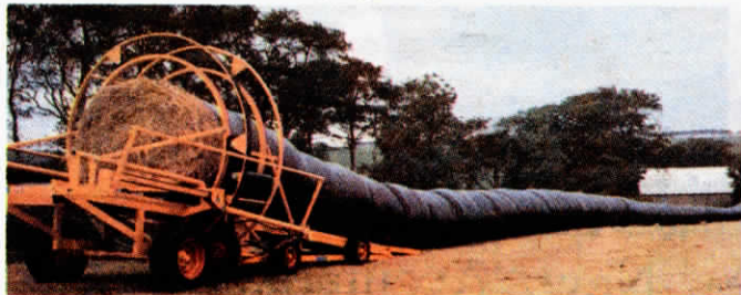
Only the outer circumference is wrapped, which cuts usage of plastic in half.
