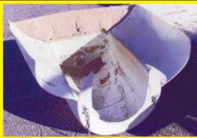
I came up with a cheap, easy way to make my own grain auger hopper. All I used was a 55-gal. plastic barrel, two short lengths of light chain, a 5/16-in. dia. redi bolt or light chain boom, and a piece of 10-in. rubber belting.
