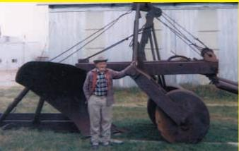
I thought your readers would like to see this 1-bottom moldboard plow that my dad and a friend, Dean Myers, built back in 1951. They designed it to plow under sand deposited 3 to 5 ft. deep on bottom land after a big flood on the Kansas river. The unit plows 62 in. deep with a 24-in. wide cut. At first they used three HD-10 bull dozers to pull the plow. Later on Myers bought a HD-19, the largest bull dozer available at that time, which allowed them to pull the plow with only two dozers.
