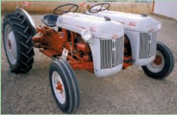
The two 8N's sit side by side on a single set of front and rear axles.
