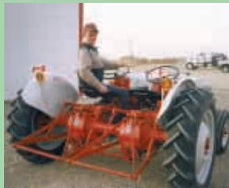
The differentials and transmissions from both tractors were left intact.
