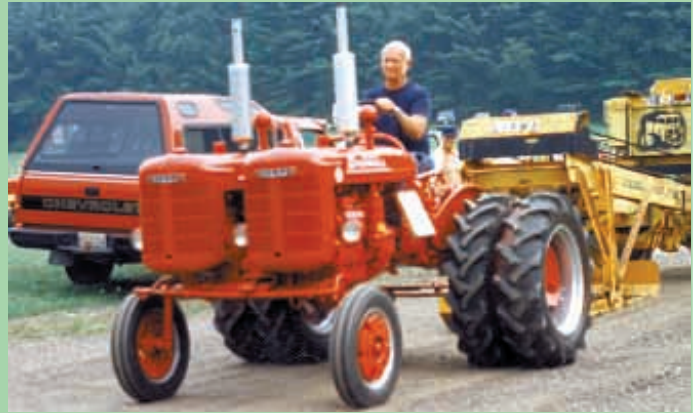
Clare Kerns put two A Farmalls on the same rear end. The tractor can be powered by either engine, or both.
