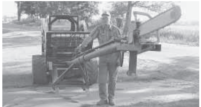
Skid steer-mounted, hydraulic-operated chain saw mounts at end of 18-ft. long boom.
