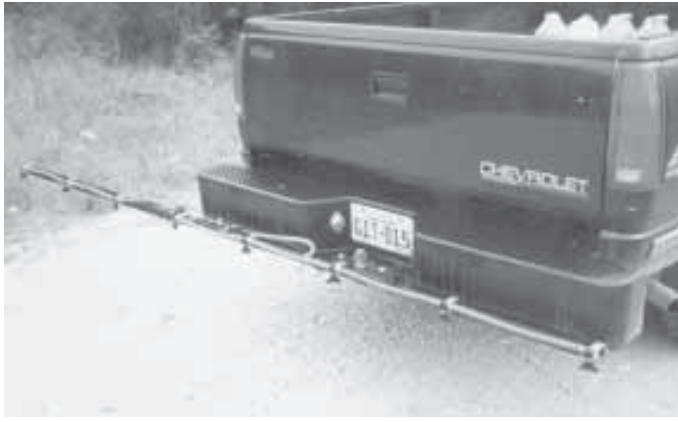
Bumper-mounted boom is supplied by a 25-gal. tank that mounts in pickup bed. Main boom measures 78 in. long while the fold-up wing boom is 47 in.
