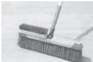
McGregor attached an 8-in. wooden scrub brush and a 7-in. piece of 1-in. aluminum angle iron to top of an 18-in. brush broom.
