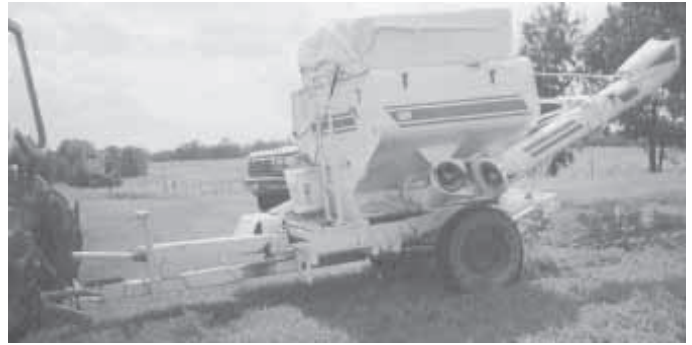
To make feed wagon, Snellings welded two Deere 55 combine grain tanks together.
