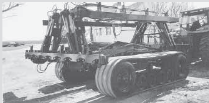
Pull-type track system is designed to fit everything from wagons to planters.
