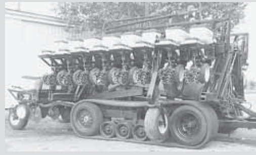
Track system designed for big planters "greatly increases flotation," says the company.
