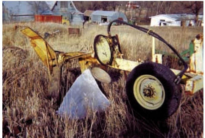
TenHulzen's "paddlewheel terrace plow" has a 3-ft. share that loosens soil up to 10 in. deep. Above the share is a short moldboard that drops soil onto a paddlewheel, which throws soil up onto the top of terrace.
