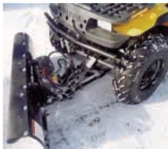
Kit bolts onto front part of blade mounting frame. It includes an electric/hydraulic power unit, a small hydraulic cylinder, and wiring.
