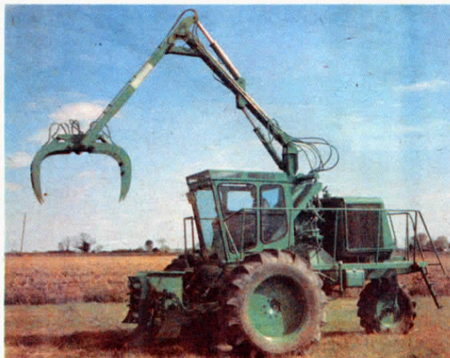
Willett converted a Deere 6600 into a 3-wheeled loader with great maneuverability and visibility.
