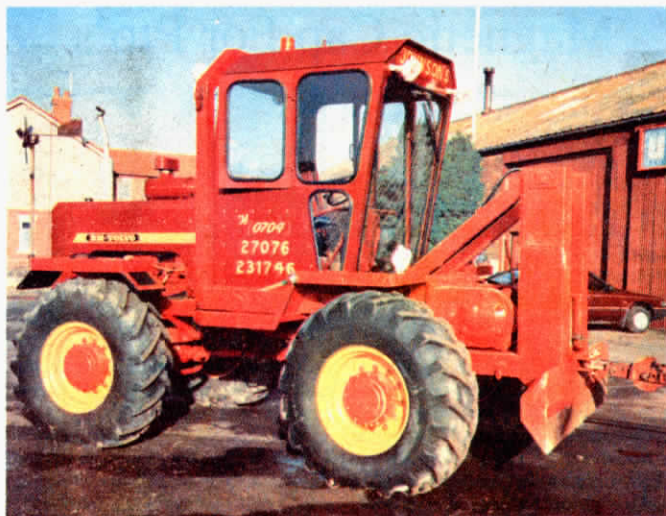
The up-front anchor blade can be driven into the ground as far as necessary when pulling with the big hydraulic winch, located just behind the anchor blade.
