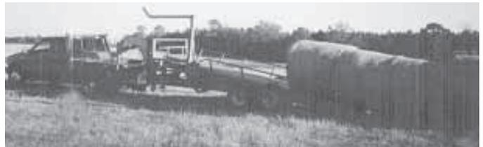
To unload bales, operator can run bales off the back one at a time or unload all bales at once by pulling on a rope to release a catch.
