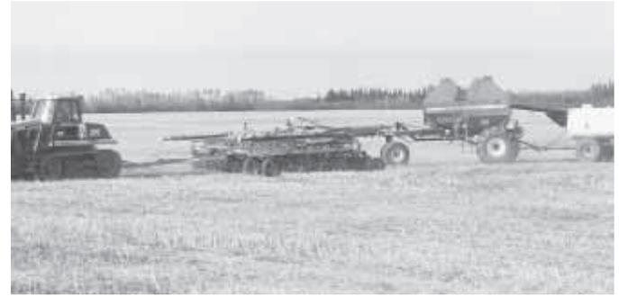
Zero-till system consists of a Cat Challenger, 50-ft. Morris Maxim Air Drill with a 300-bu. combination fertilizer/grain tank, and a 2,000-gal. anhydrous tank on back.
