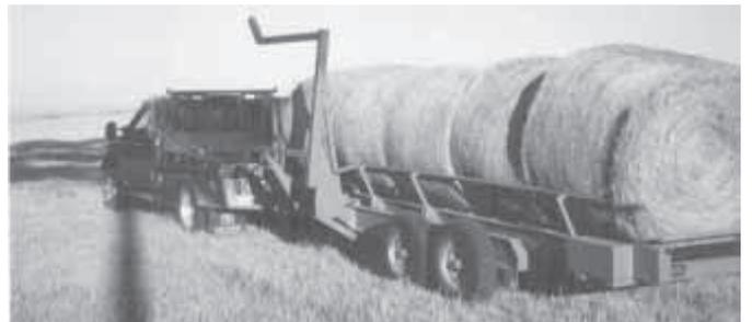
Trailer is equipped with a side-mounted loading arm and a 40-in. wide rubber belt that runs along trailer's floor. A toggle switch is used to move belt forward or back.
