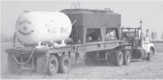
The Allard's large-scale nurse unit consists of a 35 by 8-ft. trailer carrying 2 and 4-ton hoppers and a 2,000-gal. anhydrous tank.
