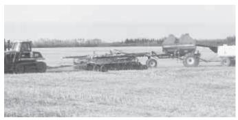
Zero-till system consists of a Cat Challenger, 50-ft. Morris Maxim Air Drill with a 300-bu. combination fertilizer/grain tank, and a 2,000-gal. anhydrous tank on back.
