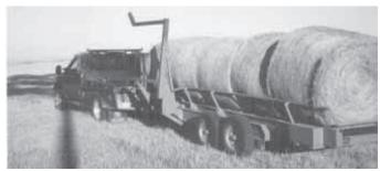
Trailer is equipped with a side-mounted loading arm and a 40-in. wide rubber belt that runs along trailer's floor. A toggle switch is used to move belt forward or back.
