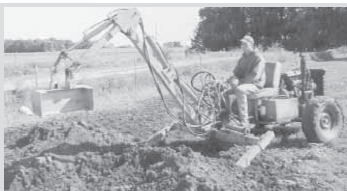
Seventeen-year-old Jason Hellickson built a full-size backhoe following commercial do-it-yourself plans. Backhoe uses bucket to pull itself along.
