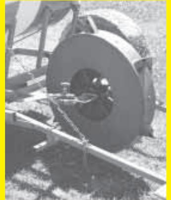
“Water wheel” planter has a 24-in. dia. steel wheel on back fitted with points that poke through plastic. Water is gravity-fed through a hose into open side of wheel.
