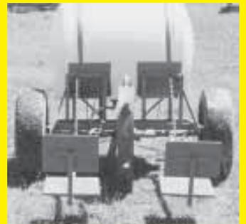
Planter is equipped with two seats, one on each side of wheel.
