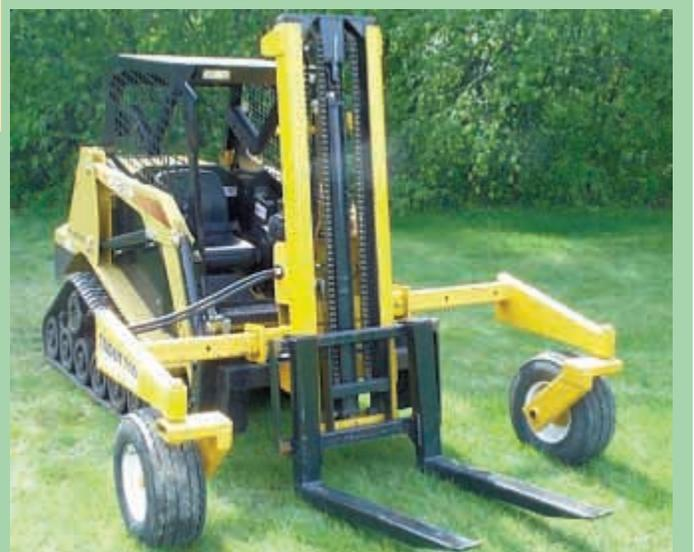
Two-wheeled mast attaches to skid steer loader arms. It uses a pair of hydraulic cylinders, and a chain-drive pulley system, to lift loads on a pair of 4-ft. forks.
