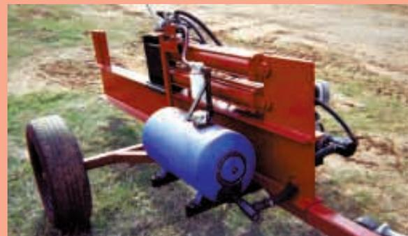
A ram, powered by twin hydraulic cylinders, forces wood chunks through stationary wedge.
