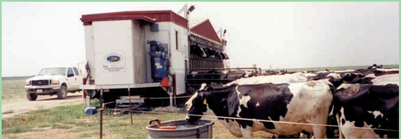
Milking parlor mounts on a 16-wheel trailer that's 65 ft. long, 12 ft. wide and 12 ft. high. Cattle are milked in a "cage" that hydraulically raises 4 1/2 ft. for easy access by workers.
