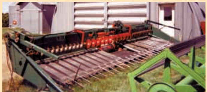
To build the unit, he merged a used Co-op 66 swather and the center part out of an old International Harvester 914 header.
