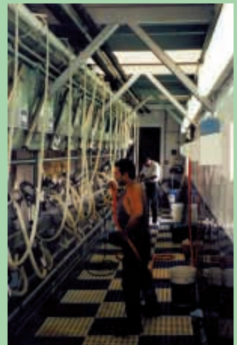
"Our portable milking parlor has everything you'd have in a conventional parlor, including milk-sensing automatic take-offs," says inventor Mark McAfee.
