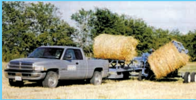
"Bale Flipper" uses an arm to load bales onto a separate trailer to which it is attached.
