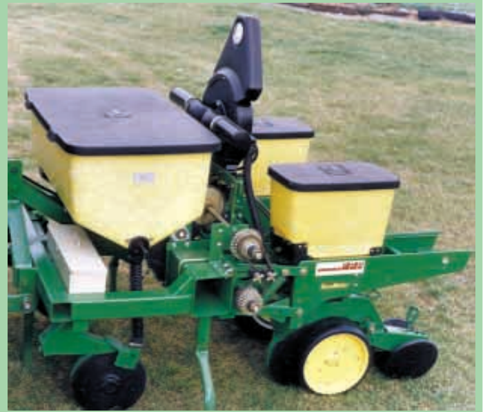
Gideon Stoltzfus builds 2 and 3-row planter frames fitted with latest Deere technology.
