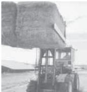
Tractor's Freeman squeeze mast is shown here with two 4 by 4 by 8-ft. bales, but it can actually handle four bales at once.
