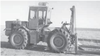
Kalcevic and sons mounted a forklift mast on back of an old Wagner articulated 4-WD tractor and turned the cab 180 degrees so the operator faces the rear.
