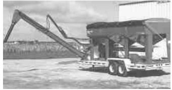
Seed handler holds the equivalent of 300 50-lb. bags of seed and can fill a 30-ft. drill in about 7 minutes. Swing away belt conveyor handles seed gently.
