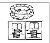
Heavy-duty washers come in two pieces and are designed to maintain enough tension on bolts and nuts to prevent loosening due to vibration or shock.
