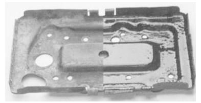
When POR-15 is painted onto rusty surfaces, it chemically reacts with the rust to create a rock-hard finish that won't crack, chip, or peel.
