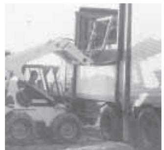
He uses a skid loader and a Steffen 15-bale grapple fork to load bales over side of trailer.
