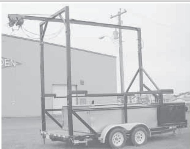
Trailer is used to prepare animals for butchering and then bring them back to a meat locker plant. Overhead trolley beam drops down for transport.
