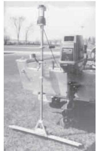
Battery-operated, “Weedsickle” mounts on a boat and cuts weeds growing under water before they go to seed.
