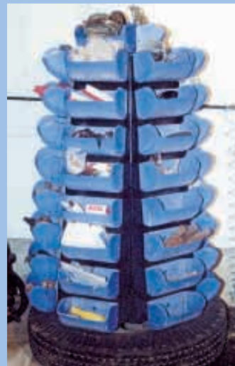
Arvin De Cook made this "nuts and bolts holder" out of plastic grain elevator buckets. "What's nice about this setup is that I can put it in the corner of my shop without taking up a lot of wall space," he says.
