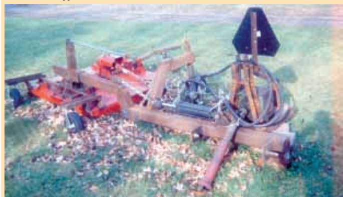
Mower is pto-driven off a right angle gearbox and is raised or lowered by a hydraulic cylinder that has a length of chain attached to it.
