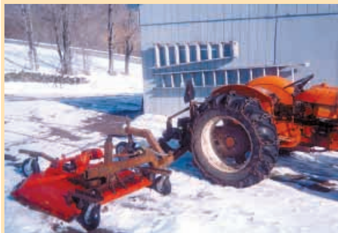
James Finch built this 3-pt. mounted hitch that lets him use his 4-ft. Bush Hog mower on roadside ditches and stream banks. Hitch hinges in middle so it flexes up or down.
