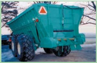
Heavy duty, 5-ft. wide apron chain at bottom delivers manure to a beater on back, which spreads manure in a pattern about as wide as the wheels.
