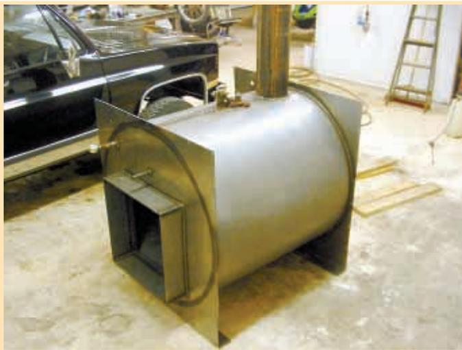
Kit comes with steel parts already cut out. The buyer welds them together. Available in regular plate steel or stainless steel.
