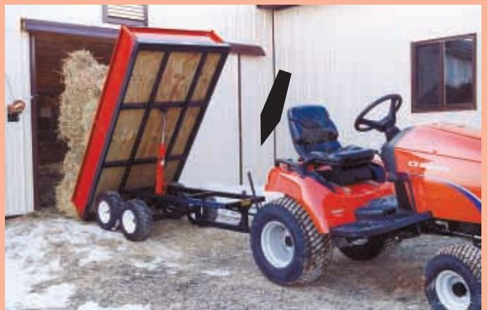
Trailer is dumped by a 3-ton, 30-in. hydraulic cylinder powered by a hand-cranked bottle jack. To dump load, Nolt simply pumps the handle (see arrow) on trailer tongue.
