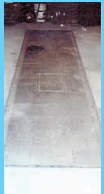
Service pit is equipped with retractable hydraulic floor. When it's not needed, the hydraulic-controlled floor is raised so it's level with shop floor.
