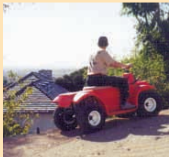
All-electric "Gorilla" ATV rides on heavy duty Dana axles and differential. On-board charger plugs into standard 110-volt outlet.
