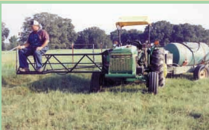
Godwin made a boom that attaches to front of his tractor and has a seat at the end. One person drives the tractor while another person does the spraying.
