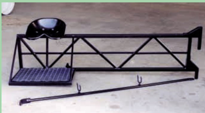
Steel seat off a Ford tractor mounts at end of boom, with a platform below it made from expanded steel mesh.
