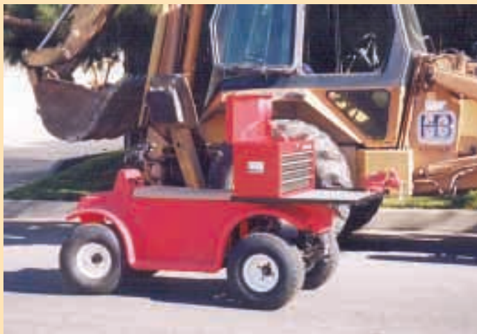
Unit is powered by electric motors that are similar in operation to those found on golf carts, but with much higher torque and speeds.
