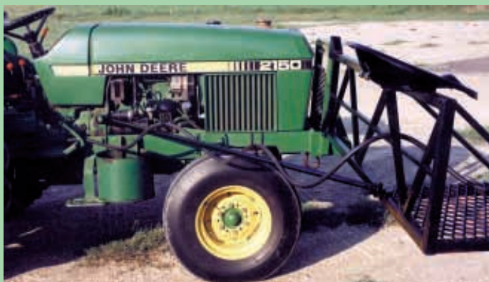
Boom was made out of two equal lengths of 1 1/2-in. thin-walled sq. steel tubing, with cross pieces welded between them at an angle.
