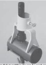
Align-O-Let welding jig can be used on pipe from 1/2 to 2 in. in diameter.
