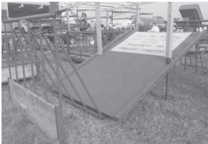
Fenceline feeder holds two bales. It's sold as a kit that consists of a steel pipe frame and brackets.
