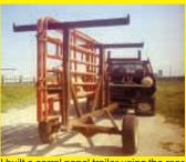
I built a corral panel trailer using the rear axle off an old pickup and some other odds and ends. It's much easier hauling the panels on a trailer than it would be on a truck or with a front-end loader.
